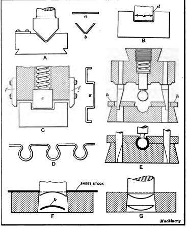
Fig. 1. Simple Types of Bending Dies
